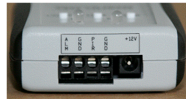
VIR-50 terminal with PIR IN and dual activation ALARM OUT
